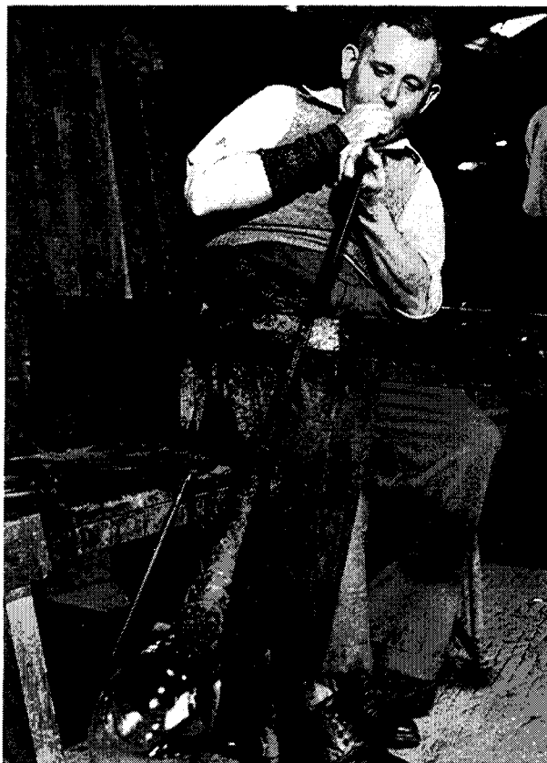
A molten bubble of glass extends from the end of the blowpipe as a glass blower forms the initial shape of a vase.
